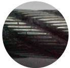
Crown breaks on a compacted rope
