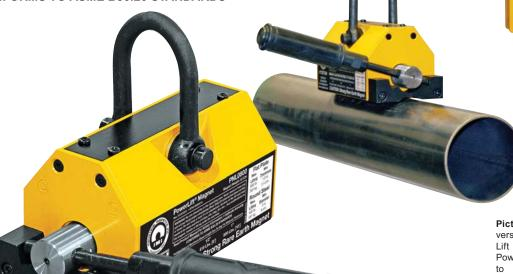
Picture above: A customized version of IMI's Vertical Lift Adaptor featuring two PowerLift® magnets, designed to lift ferrous metal from horizontal to vertical orientation or vise versa. Adjustable for various widths, thicknesses and shapes. Ask for Tech Sheet MG-02G for specifications.
