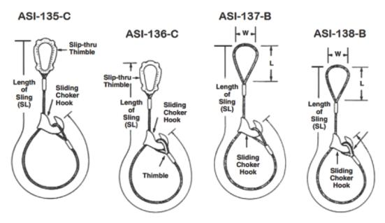
Sling #135 is similar to #136, but has a spliced loop on the load end in place of a thimble.
